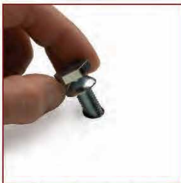
1 Insert Shear Bolt into application
