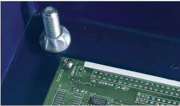
Placing fasteners in tight corners makes access for impulse tampering harder.
