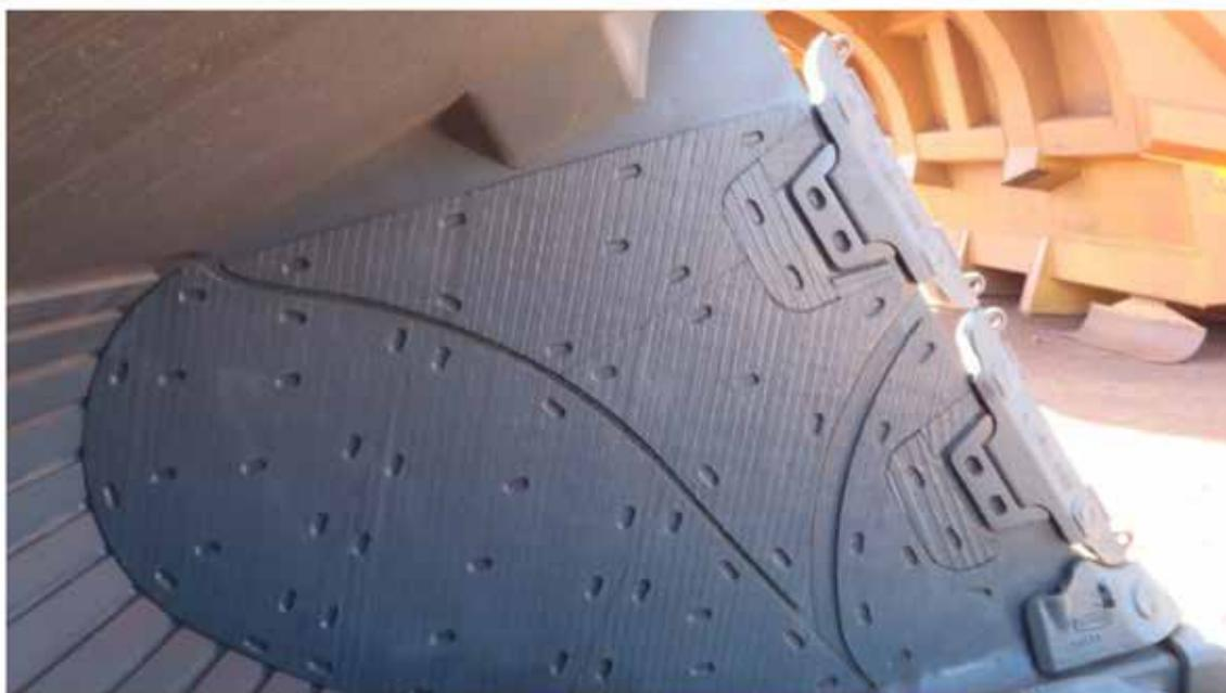
PACplate, our leading chromium carbide clad wear plate, delivers superior resistance to wear in any operating condition. Using the latest manufacturing technology, PACplate is proven to deliver industry benchmark wear resistance as tested using ASTM G65 wear testing, plus leading resistance to impact failure. Our testing shows the PACplate can withstand over 6 times the impacts that would deliver a central failure, and over 25% more impacts prior to edge failure.
